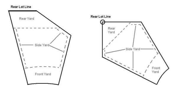
Figure 2-4: Illustration of Rear Site Lines
