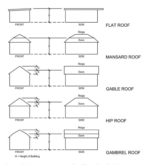
Figure 2-1: Interpretation of Building Height Measurement
