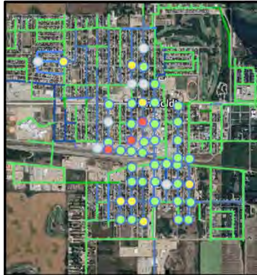
Leak Detection Sensor Program Screenshot
